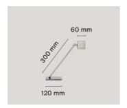
on plug, base in pressofused zamak. Directionable head. ON/OFF switch with Soft Touch technology and light flow adjustment to 2 intensities (100% -50% – 0%). Power pack on plug with interchangeable plugs.
