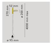
or chromed die-cast aluminium. Directionable head. The light fitting can be moved vertically by running the internal structure of the body on a steel cable tensioned between the ceiling and the floor (useful length 4000mm). Dimmable switch with Soft Touch technology. Adaptor on plug connector with interchangeable plugs.
