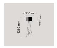
polished and chrome-plated Zamak alloy. Injection-molded PA6 (nylon) lamp-cover. Color: white. Injection-molded PC (polycarbonate) inner diffuser. Color: 3% opal. Injection-molded elastic PVC (polyvinylchloride) feet. Lathe-shaped aluminum diffusers, painted white on the inside, and shiny white or black on the outside or gray-colored, blown and overlaid glass with glossy external finish. On the cable there is the electronic dimmer which allows the regulation of light brightness.
