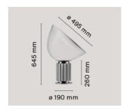
Directionable diffuser in transparent PMMA. Body in matt black or naturally anodized extruded aluminium. Base in nickel-plated metal. Electric cable of useful length 220 cm, with dimmer switch for ON/OFF and adjustment of the light flow between 10-100%. Plug-in power supply with interchangeable plugs.
